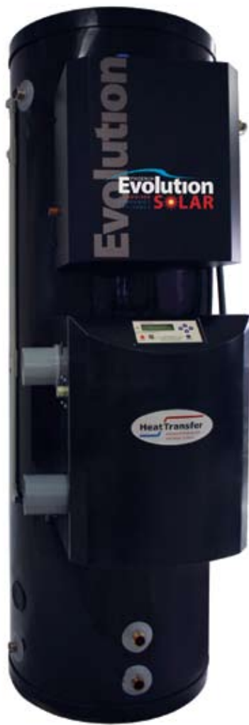
Heat Transfer Products' Phoenix Evolution incorporates a modulating condensing water heater and a module that draws heat from the water for use in space heating applications.
